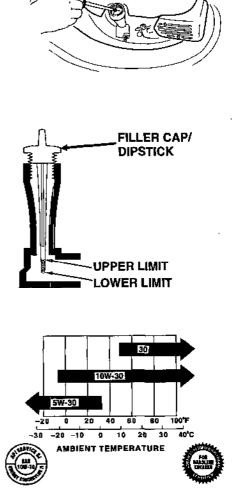
The SAE oil viscosity and service classification are in the API label on the oil container. Honda recommends that you use API SERVICE category SH or SJ oil with the ILSAC "starburst" certification mark displayed on the container.
