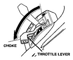
Move the throttle lever to the FAST position. The choke arm should move clockwise, until it contacts the stop post on the carburetor.
