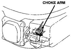
3. If the choke arm does not move all the way to its stop, in either direction, take the mower to an authorized Honda servicing dealer. Throttle cable adjustment involves related control plate adjustments.
