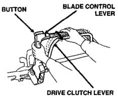
When moving and using the drive clutch lever to change self-propelled speed, continue to fully hold the blade control lever against the handlebar. This will help to extend the service life of the blade control mechanism.
