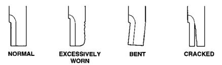
A dull blade can be sharpened, but a blade that is worn out, bent, cracked, or otherwise damaged must be replaced. A worn or damaged blade can break, causing blade pieces to be thrown from the mower.
