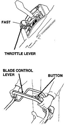
Always release the blade control lever before starting the engine to prevent the blade from turning.
