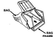
2. Clip the plastic edges of the bag onto the frame, as shown.
