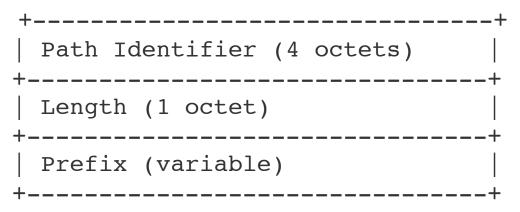
Path Identifier can be used to prevent a route announcement from implicitly withdrawing a previous one
