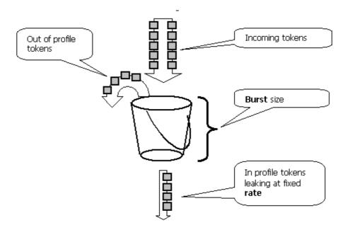
**Note:** The traffic is not buffered in the bucket as it can appear in this example. The actual traffic does not flow through the bucket at all; the bucket is only used in order to decide whether the packet is in profile or out–of–profile.
