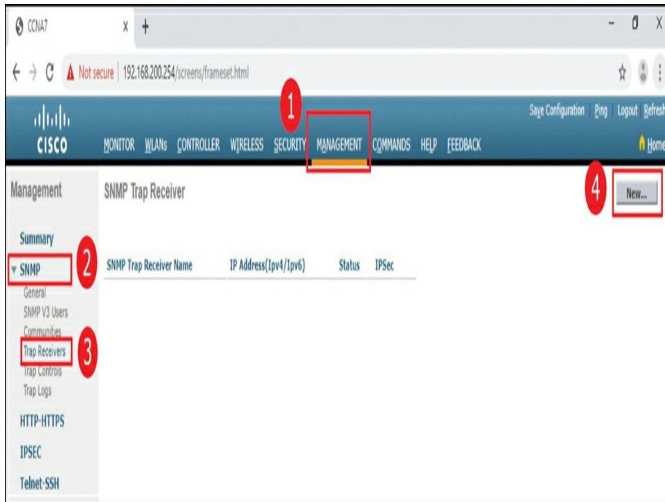
Figure 13-33 Creating a New SNMP Trap Receiver
