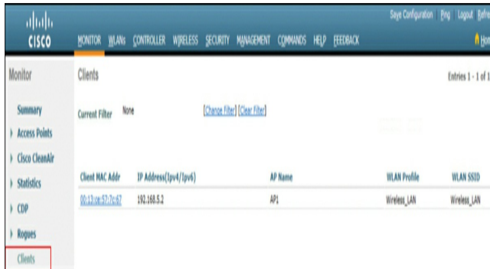
Figure 13-31 View Wireless Client Details
