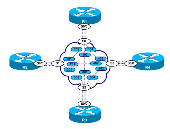
Provided below is the Frame-Relay switch configuration. If you enter this configuration into a router acting as a Frame-Switch and you cable up your pod in the manner displayed on this page, you will have configured a full-mesh Frame-Relay topology.
