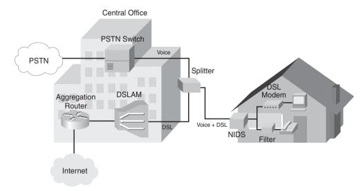
Recall that DSL is a Layer 1—Physical Layer—technology. Following are the three methods of carrying data at Layer 2 over DSL:
