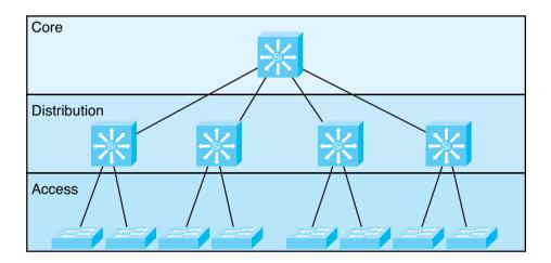
This is a simple drawing of how the three-layer model might be built out for a campus network. A distribution Layer-3 switch is used for each building on campus, tying together the access switches on the floors. The core switches link the various buildings together.
