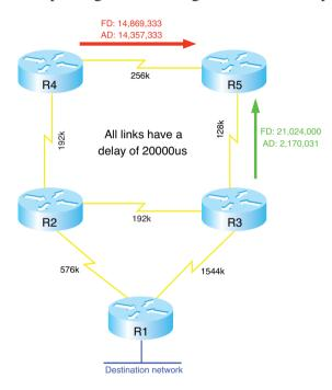
How does R3 choose its path? Figure 2-4 shows the path selection process for R3.
