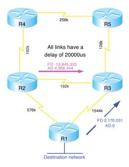
R1 will be its successor because it has the lowest metric. However, no feasible successor exists because R2's AD is greater than the successor path metric. If the direct path to R1 is lost, R3 has to query its neighbors to discover an alternative path. It must wait to hear back from R2 and R5 and will ultimately decide that R2 is the new successor.
