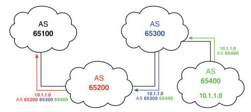
Use BGP when the AS is multihomed, when route path manipulation is needed, or when the AS is a transit AS. (Traffic flows through it to another AS, such as with an ISP.)
