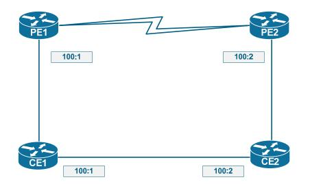
In this case, if PE1 redistributes a prefix into MP-BGP it will be tagged with 100:1. The prefix will reach PE1 and pass down to CE2. The prefix will finally be stopped at CE1 by SoO filtering and will never loop back to PE1 again. The same applies to prefixes redistributed into MP-BGP by PE2.
