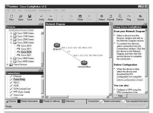
Figure 6-4 Cisco ConfigMaker tool for network design and implementation
