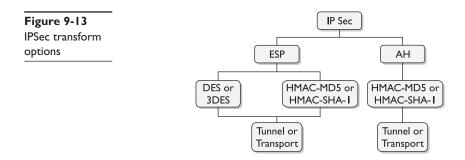
The actual transforms supported might vary by device type. VPN devices support a slightly different group than the PIX Firewall. The following are transforms supported by the IOS-based devices.
