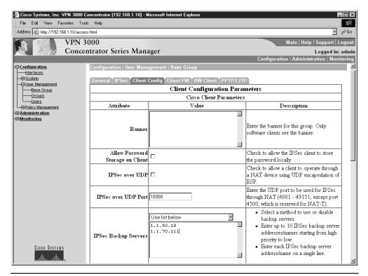
Figure 15-26 Configure backup servers on the VPN Concentrator
