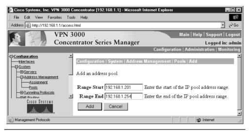
Figure 14-19 Defining a pool of addresses for remote users to use
