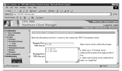
Figure 15-25 Configure backup servers directly on the VPN 3002 Client
