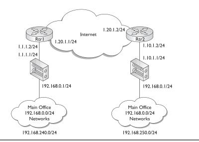
Figure 16-15 Overlapping network address scenario
