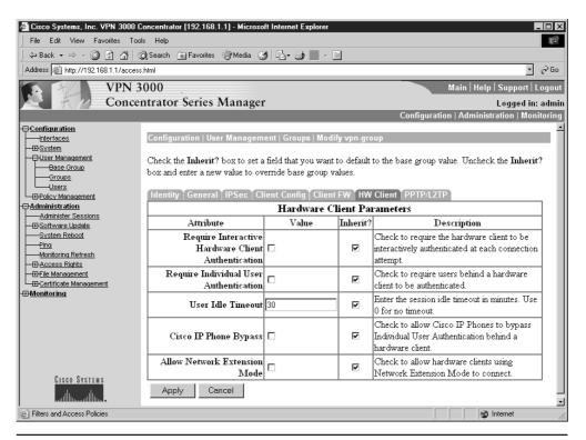
Figure 14-29 Group parameters screen showing the Inherit option
