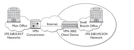
Figure 15-29 VPN scenario network with the main office using RRI
