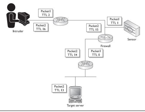
Figure 23-2 Manipulating network-based sensors using TTL
