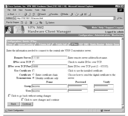
Figure 15-18 IPSec configuration screen
