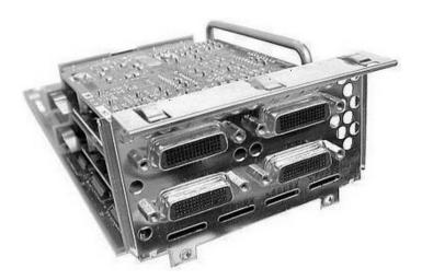
At the top end, the AS5x00 series routers can support dozens to thousands of outside connections in a variety of combinations. The AS5400 and AS5800 routers provide the capability to terminate ISDN, 56K analog modem, fax, and VoIP calls on the same interface. The AS5400 can support over 600 connections, while the AS5800 can support 2,000.
