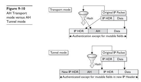
In *AH Tunnel mode*, the entire original IP header and data becomes the "payload" for the new packet: a new IP header reflecting the end points of the VPN tunnel is added and the hash is performed on the resulting packet. The new IP header is protected exactly the same as the IP header in Transport mode. The fields that change in transit are excluded. The hash result again becomes the AH header following the new IP header.
