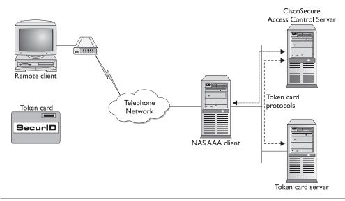
Figure 4-4 Remote user authentication using Token Card
