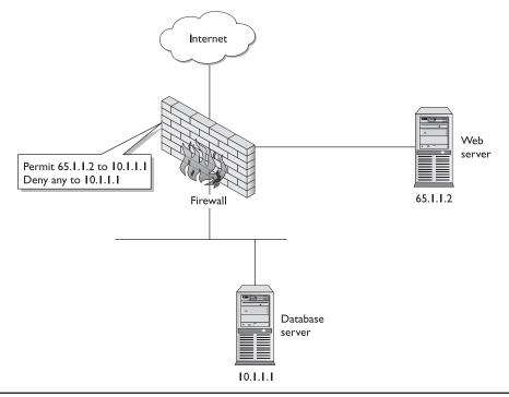
Figure 23-1 Attacking IP trust relationships between compromised hosts
