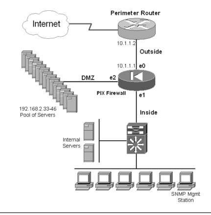
Figure 20-1 SNMP management station in the inside network
