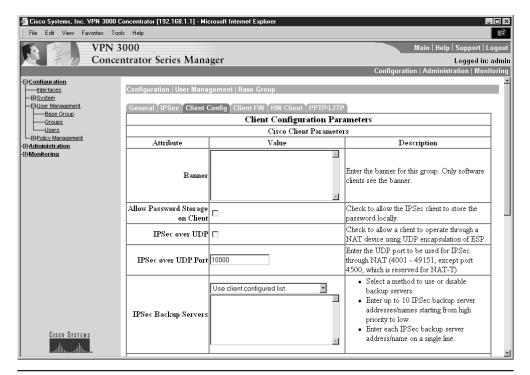
Figure 16-14 Configuring IPSec over UDP on the Concentrator
