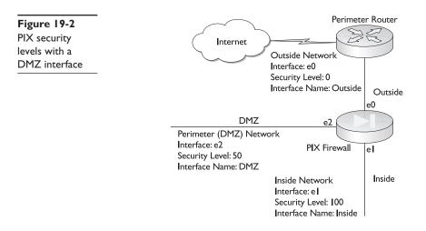
originating from the inside interface could flow freely to the DMZ and reply packets could return to the inside interface. Packets originating in the DMZ that aren't a part of a session originating from the inside interface, couldn't travel to the inside interface without configuration assistance.
