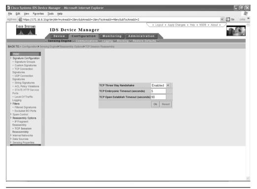
Figure 25-21 TCP reassembly configuration pane
