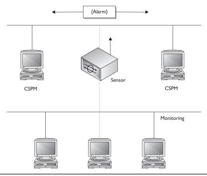
Figure 24-5 Reliable message delivery via the PostOffice protocol
