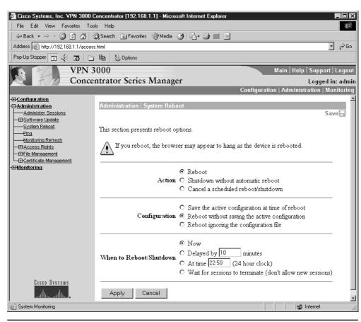
Figure 14-49 System reboot and shutdown options
