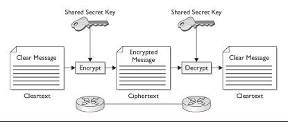
Figure 9-7 DES encryption process
