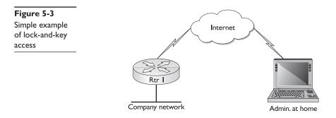
**The Dynamic ACL Statements** The dynamic access list feature is an option for both numbered and named extended access lists for TCP, UDP, ICMP, and IGMP traffic. The [dynamic *dynamic-name* [timeout *minutes*]] options precedes the {permit | deny} choice.
