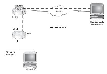
Figure 21-2 IPSec remote access VPN implementation (transport mode)
