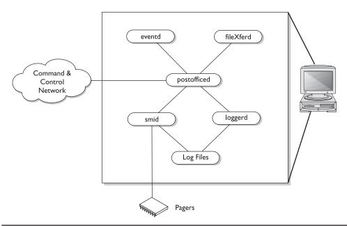
Figure 24-10 CIDS sensor architecture
