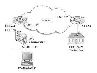
Figure 14-12 VPN Concentrator remote access scenario
