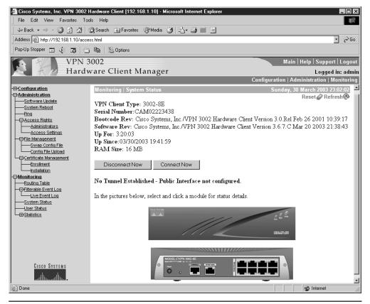
Figure 15-10 Web interface displaying system status
