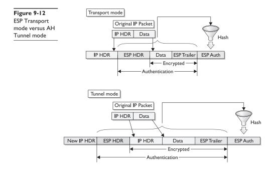
In ESP Tunnel mode, as in AH, a new IP header reflecting the end points of the VPN tunnel is added. Both encryption and authentication incorporate the entire original IP header.
