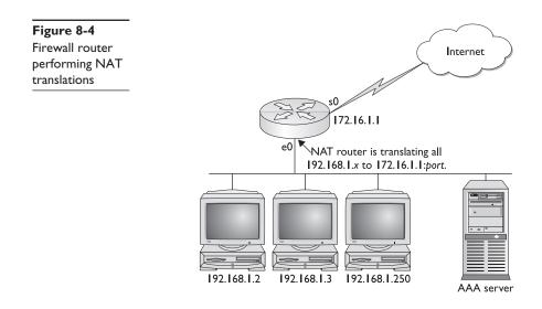
occur outbound after the traffic has passed through the LAN interface, everything should be okay so far. The NAT translations on returning traffic shouldn't be an issue because the returning traffic is unfiltered outbound on the LAN interface. Even if the traffic was filtered, the addresses have been retranslated back to the local addresses before heading out into the LAN.
