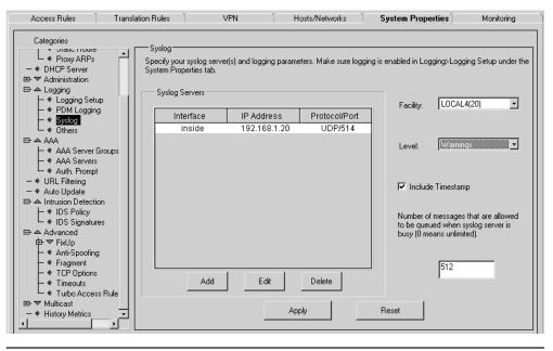
Figure 22-7 Configuring a Syslog Server with PDM
