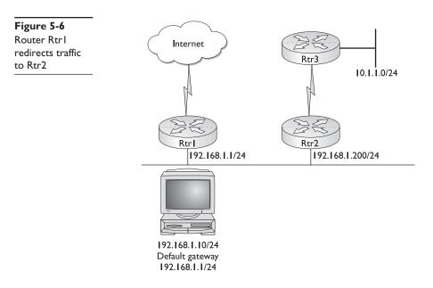
By default, Cisco routers send ICMP redirects. You can use the interface subcommand no ip redirects to disable ICMP redirects. Another solution is to use an ACL to filter out any incoming ICMP redirects. The following code contains examples of each:
