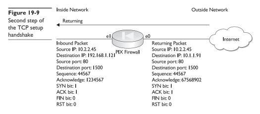
Note that both the SYN and ACK flag bits are on, which indicates this is the second step in the handshake. If both the SYN and ACK flag bits aren't on, the packet will be dropped for not being the next expected step. The SYN bit is on because host 10.2.2.45 is supplying its synchronization number to the local host.
