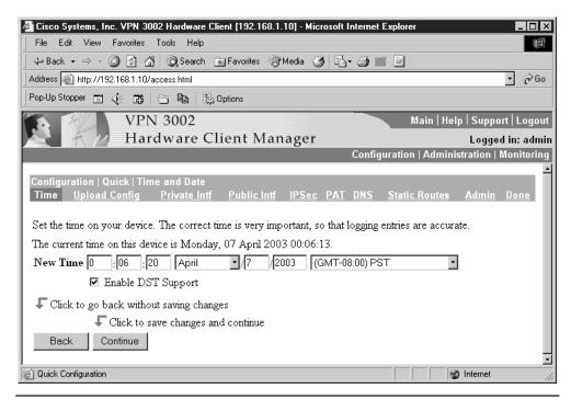
Figure 15-13 Screen to set date, time, and time zone for the device
