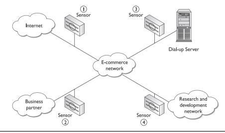
Figure 25-1 Sensor deployment at network entry points
