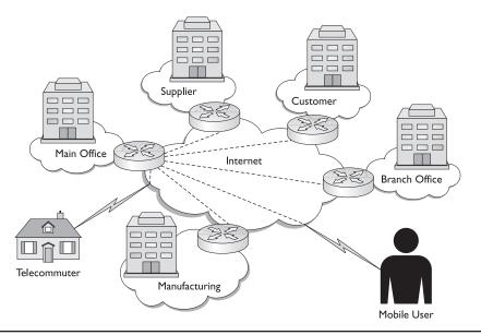
Figure 9-9 Typical Tunnel mode VPN connections
