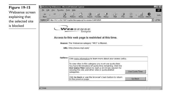
Websense protocol enables group and user name authentication between a host and a PIX Firewall. The PIX Firewall performs a user name lookup, and then the Websense server handles URL filtering and user name logging. User name logging tracks the user name, group, and domain name on the Websense server.
