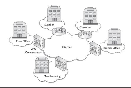
Figure 14-11 LAN-to-LAN VPN connection example
