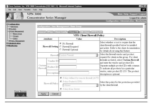
Figure 14-25 Defining client firewall default requirements
