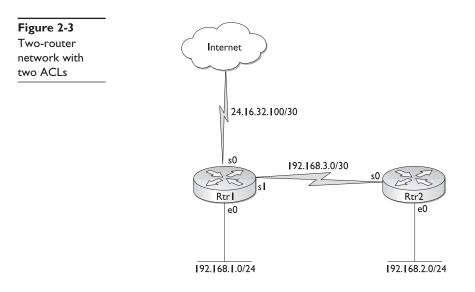
The first line of ACL 20 permits host (192.168.2.20) from the Rtr2 LAN to access the LAN on Rtr1. The second line blocks the rest of 192.168.2.0 subnet mask 255.255.255.224, or addresses 192.168.2.0 to 192.168.2.31 from the Rtr1 LAN. The final line allows the rest of Rtr2 LAN and anything coming in over the Internet.
