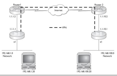
Figure 21-1 IPSec site-to-site VPN implementation (tunnel mode)
