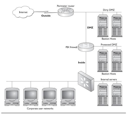
Figure 5-1 Network design with perimeter security
