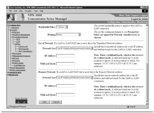
and enter **0.0.255** in Wildcard Mask field. In the Remote Network section, enter **192.168.250.0** in the IP Address field and enter **0.0.0.255** in Wildcard Mask field. Click on Apply when finished. The Vendor Concentrator would be a mirror image of these entries.
