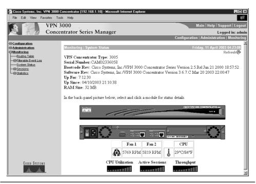
Figure 14-7 System monitoring screen
