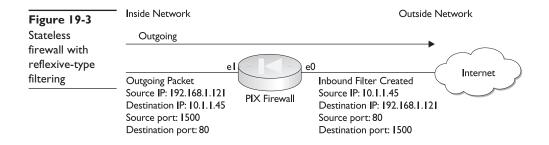
what if the original request was to an FTP server, where the packet was sent to port 20, but port 21 responds? Now the filter isn't right. Remember, firewalls are mindless devices that can only follow rules and can't interpret or be appealed to with logic. The return traffic would probably fail.
