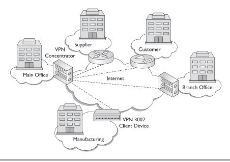
Figure 16-1 Common LAN-to-LAN VPN implementations
