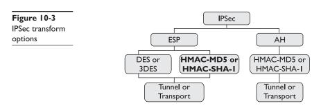
The actual transforms supported might vary by device type. VPN devices could support a slightly different group than the PIX Firewall. The following are transforms supported by the IOS-based devices:
