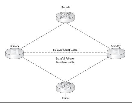
Figure 22-18 Failover system with stateful failover cable installed
