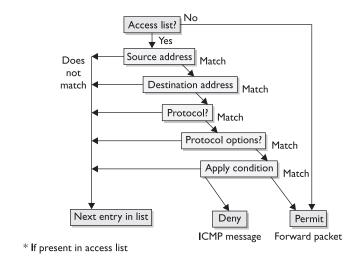
Figure A-3 Extended access list processing steps
