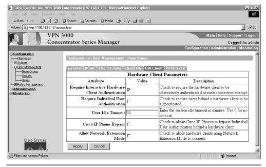
Figure 15-24 Configure Interactive Hardware Client Authentication
