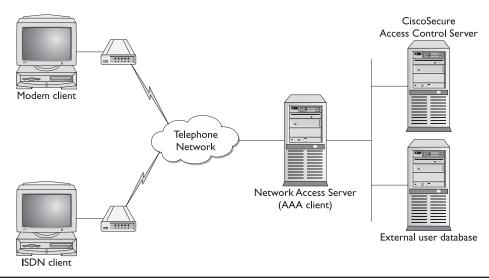
Figure 4-1 Cisco Secure ACS with an NAS AAA client
