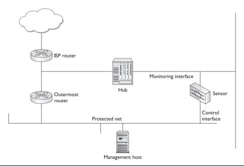
Figure 25-2 Sensor in front of a filtering device
