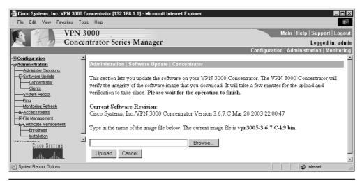
Figure 14-50 VPN Concentrator software upgrade screen
