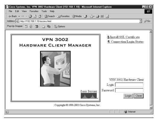
Figure 15-5 VPN 3002 Hardware Client Manager login screen
