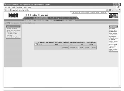
Figure 25-27 Adding a managed device
