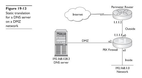
Because of the high number of attacks on DNS services, PIX Firewalls now only allow the first DNS reply to pass through, and then they drop all others. This prevents man in the middle attacks, where the attacker sends a second DNS reply, creating a bogus domain name resolution that would direct the browser to the wrong site. Unfortunately, DNS service would accept the later reply and update its table.
