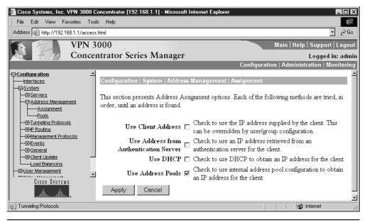
Figure 14-18 Selecting an inside address assignment method for remote users
