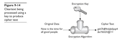
The key terms in the process include data, key, encryption algorithm, and cipher text.
