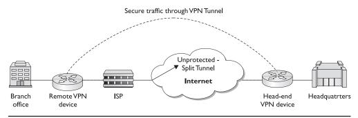
Figure 12-1 A secure VPN tunnel and split tunneling for web browsing
