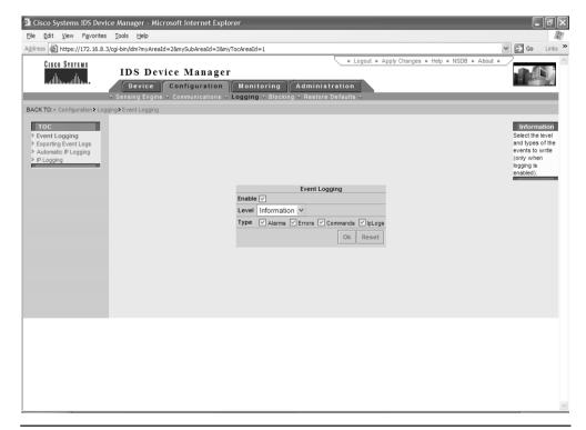
Figure 25-23 Event logging configuration panel
