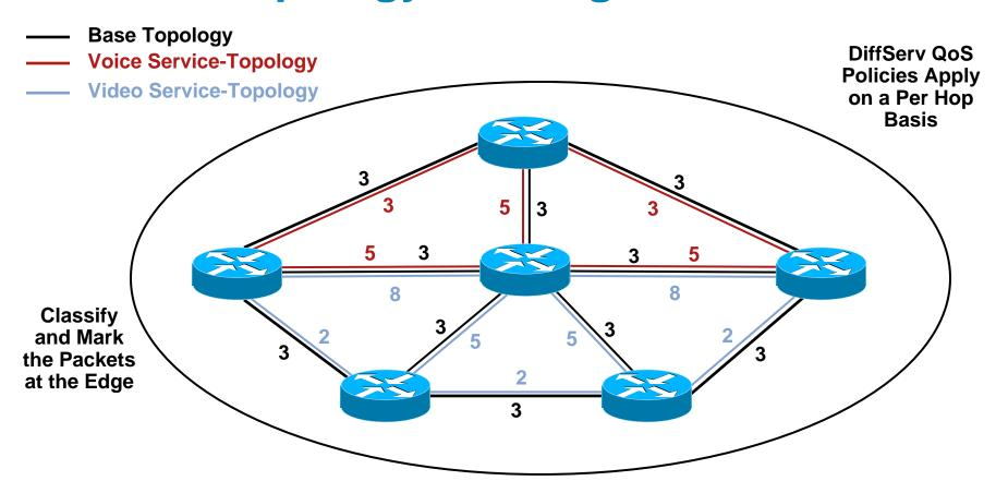
Goal: Destination Based Routing Based on Traffic Types... **Service-Topologies Are Independent Entity in Itself Each Link Can Have Multiple Service-Topologies** Multiple DSCP Values Can Be Mapped to a Single Service-Topology
