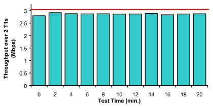
**Two full T1s.** The chart shows the actual bi-directional link loads, that the 2811 router was processing over two T1s. These were aggregated via Multilink PPP, using bi-directional connectivity between the office and the ISP's access router.
