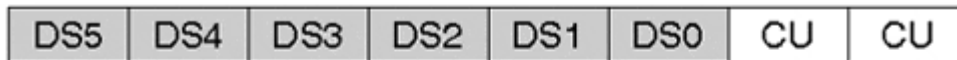
Figure G-2 Differentiated Services Code Point (DSCP) Bits in the Differentiated Services (DS) Byte
