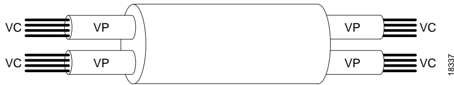
Figure 1-6 ATM Virtual Path And Virtual Channel Connections
