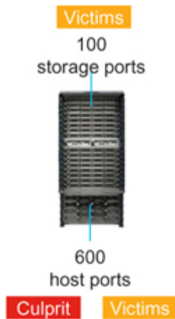
Figure 6-41 Collapsed core design with one culprit and 50 victims
