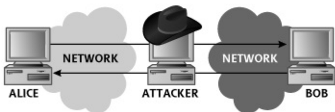
Figure 8.11. In a monkey-in-the-middle attack, the attacker can grab or alter traffic between Alice and Bob.
