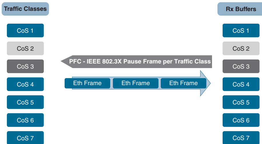
Figure 14-3 IEEE 802.1Qbb Priority Flow Control
