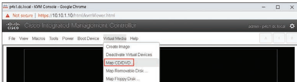
Figure 18-13 Mapping the ESXi Hypervisor ISO Image (1)
