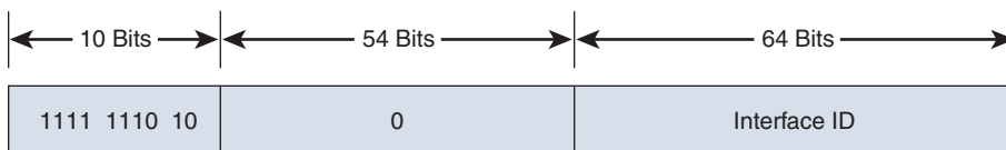
Figure 2-3 IPv6 Link-Local Address Format
