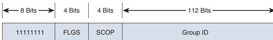
Figure 2-6 Multicast Address Format
