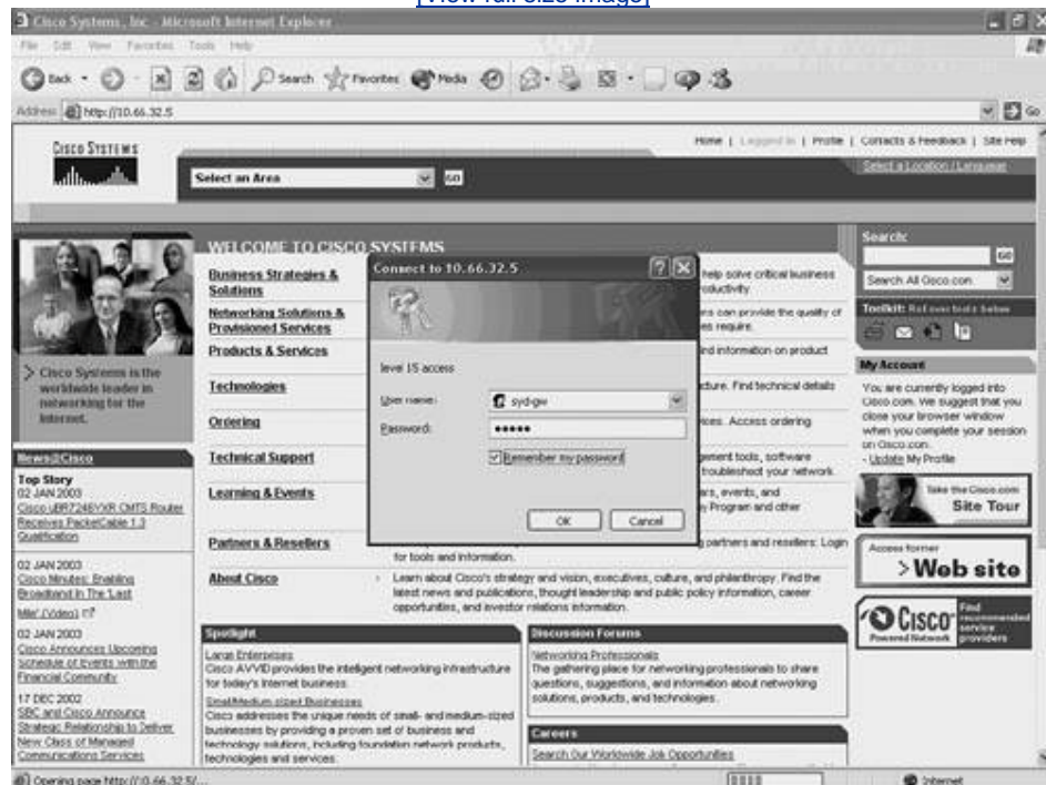
Figure 2-4. HTTP Authentication on a Cisco Router
