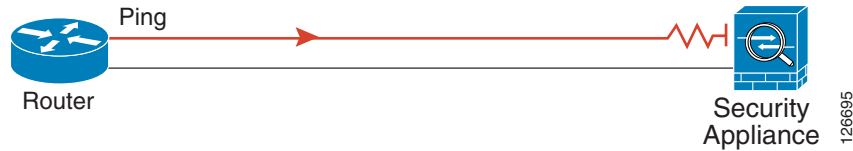
Figure 36-2 Ping Failure at Security Appliance Interface
