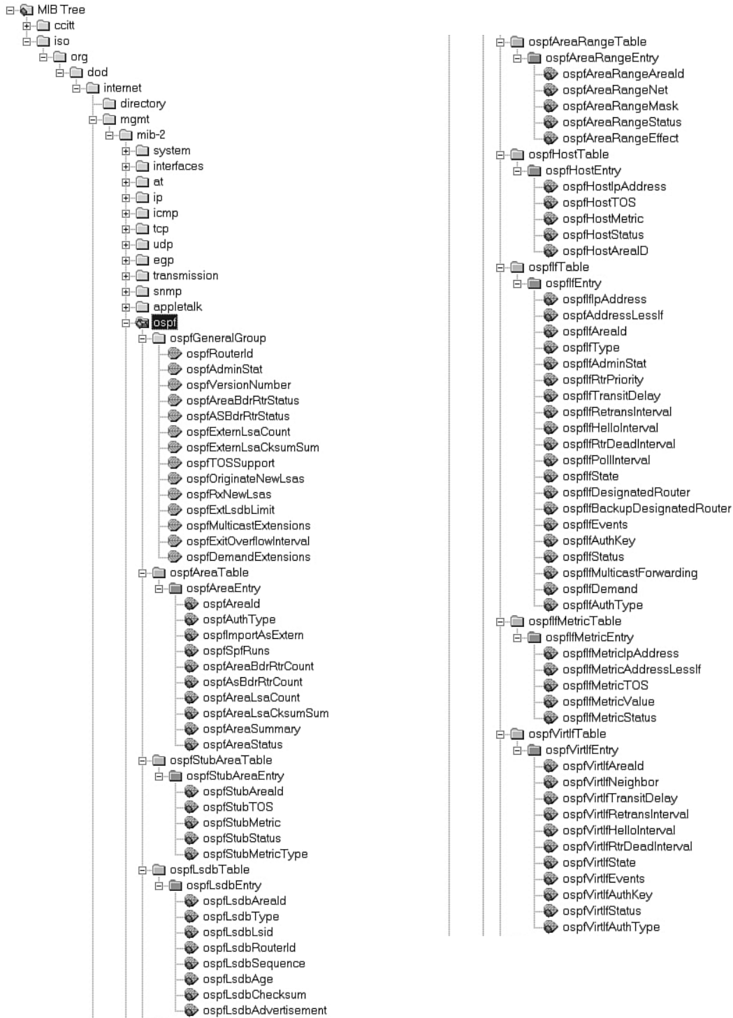
Figure 8-12 Detailed OSPF MIB Tree
