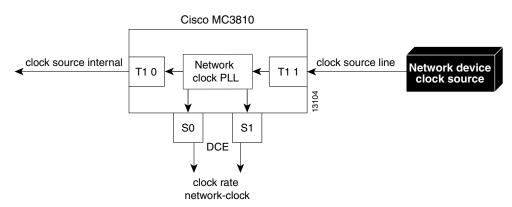
Figure 143 Obtaining the Clock Source from a Network Device Attached to Controller T1/E1 1
