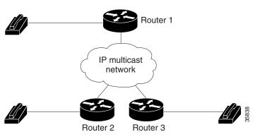
Figure 153 Cisco Hoot and Holler over IP with Frame Relay Topology
