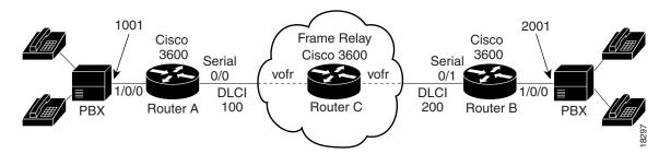
Figure 97 Tandem Configuration with Three Routers for Switched Calls
