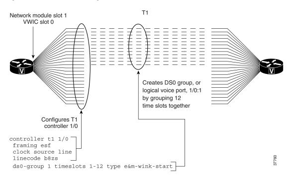
Figure 33 T1 Controller Configuration on Cisco 2600 or 3600 Series Routers
