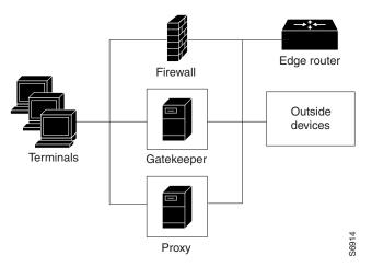
In co-edge mode, the proxy can present a security risk. To avoid exposing a network to unsolicited traffic, configure the proxy to route only proxied traffic. In other words, the proxy routes only H.323 protocol traffic that is terminated on the inside and then repeated to the outside. Traffic that moves in the opposite direction can be configured this way as well.
