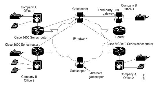
Figure 136 IP Network for T.38 Fax Relay
