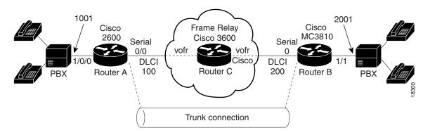
Figure 99 Tandem Configuration with a Cisco MC3810 Multiservice Concentrator Endpoint Node
