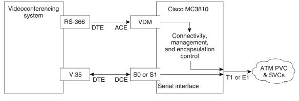
DTE=data terminal equipment DCE=data communications equipment ACE=automatic calling equipment VDM=video dialing module
