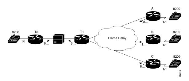
In this example, all digits matched with destination 8... are forwarded to the appropriate port. For a call from Router A to reach extension 8208, the call first terminates at Router T1, which plays out the digits 8208 to the voice port connected to the PBX. The PBX then routes the voice call to Router T2. The **forward-digits all** command is used here, but the **forward-digits 4** command could also be used in this example.
