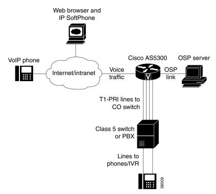
To implement VoIP authentication, the gateway must be connected to the Internet or intranet and to an OSP server. The OSP server, which can be any properly configured Windows NT or UNIX server, communicates over a Computer Telephony Interface (CTI) link to a Class 5 switch or PBX. Use the settlement command **type** and include the *uni-osp* argument to configure the UNI-OSP feature.
