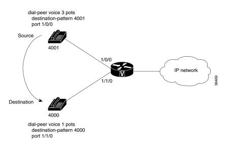
This type of configuration is similar to the configuration used for hairpinning, which occurs when a voice call destined for the packet network is instead routed back over the PSTN because the packet network is unavailable. For more information about the hairpinning feature, see the "Hunt Groups and Preferences" section on page 180.
