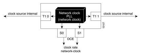
Figure 146 Using the Cisco MC3810 Internal Clock Source
