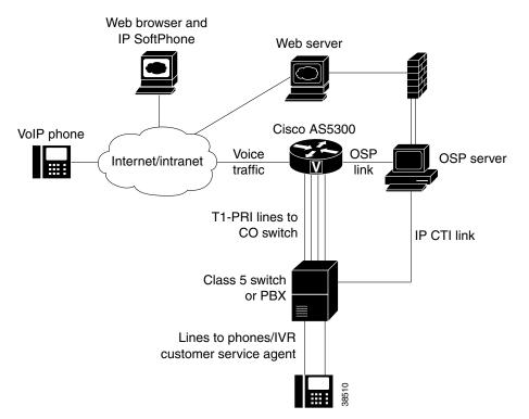
When using the click-to-talk function, a customer selects a link on a web page indicating that a request to talk to a customer service or technical support representative. The web server then launches a preinstalled SoftPhone on the web browser machine through a browser plug-in. The web server supplies the PC SoftPhone application with the telephone destination number (DNIS) of the appropriate agent, and the route point, queue, and IP address of the voice gateway.
