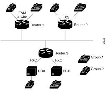
Figure 152 Cisco Hoot and Holler over IP with Ethernet Topology
