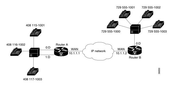
Table 18 shows the number expansion table for this scenario. The information included in this example must be configured on both Router A and Router B.
