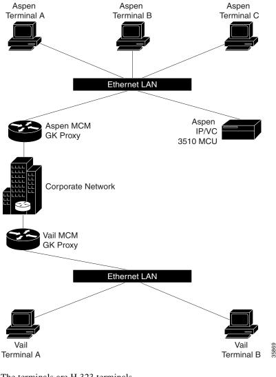
Figure 140 Interzone Calling Configuration with Two Zones
