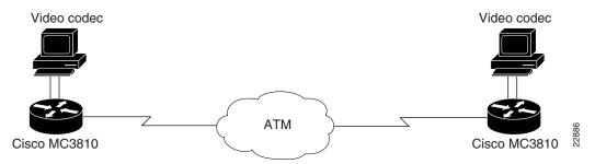
Initially, the network clocks are set up on each multiservice access concentrator so that video codecs can operate at a multiple of 64 kbps:
