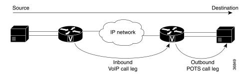
Figure 41 Call Legs from the Perspective of the Terminating Router
