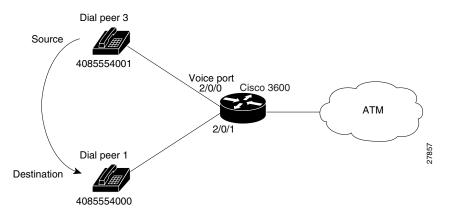
Figure 103 Communication Between Dial Peers Sharing the Same Router
