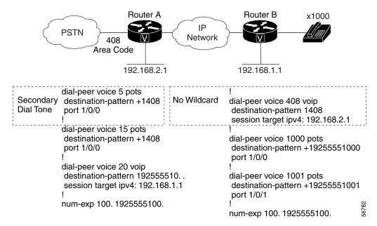
Figure 13 Cisco Two-Stage Dialing Configuration
