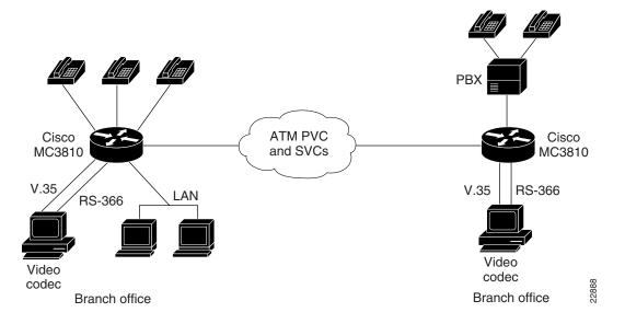
Figure 138 shows how the physical interfaces interact with software, the codec, and video data to handle connectivity and video functionality. The VDM automatic calling equipment (ACE) provides the EIA/TIA-366 interface to the video codec, and one of the Cisco MC3810 serial interfaces connects to the video codec DTE interface. The Video Call Manager (ViCM) software manages video calls that travel over a T1 or E1 facility through the Cisco MC3810 multiflex trunk (MFT) interface.
