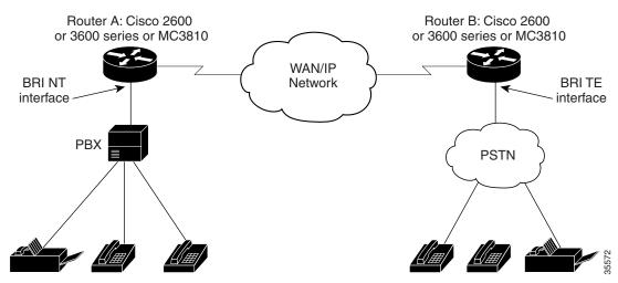
Figure 125 Typical Application Using ISDN BRI NT/TE VICs or ISDN BVMs
