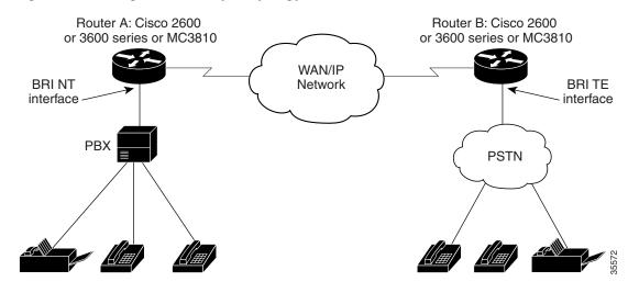
Figure 128 Configuration Example Topology
