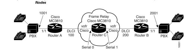
Configuration with All Cisco MC3810 Multiservice Concentrators as Endpoint and Tandem
