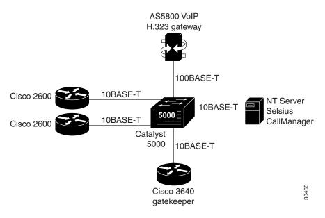
Figure 26 Cisco AS5800 Universal Access Server Acting As a Gateway
