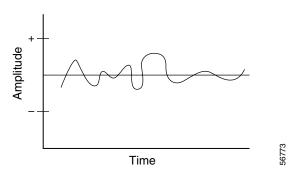
Analog signals are susceptible to line noise that distort the analog waveform and cause garbled reception. This effect is especially more obvious to the listener if many amplifiers are located between the listener and the end-office switch. Figure 6 shows that an amplifier does not clean the signal as it amplifies, but simply amplifies the distorted signal. When the signal goes through several amplifiers, the noise that is created is called cumulative line noise.
