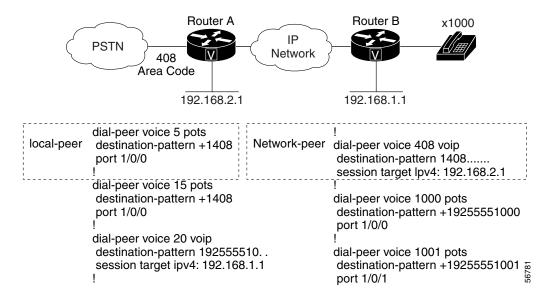
Another possibility is to use two-stage dialing. Figure 13 shows the changes to the dial plan when two-stage dialing is implemented.
