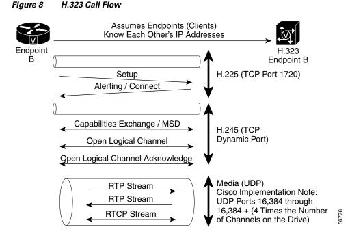
The steps required to complete an H.323 call shown in Figure 8 are as follows:
