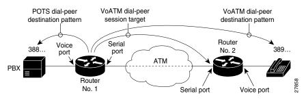
Figure 105 Relationship Between the Destination Pattern and Session Target from the Perspective of Router 2
