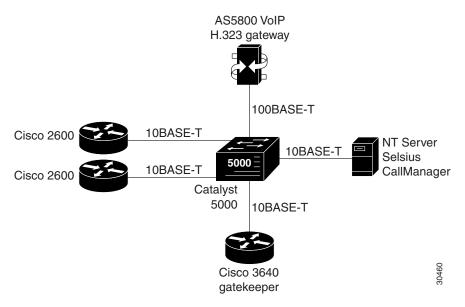
The following example shows a Cisco AS5800 universal access server configured as a gateway using RAS:
