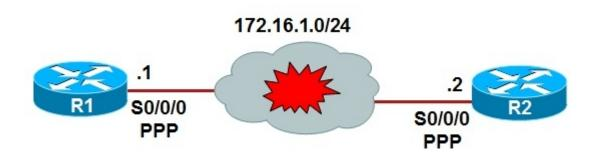
Enabling AutoQoS on R1's Serial 0/0/0 interface generates an error.
