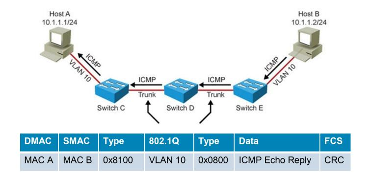
Switches forward ICMP Echo Reply unicast frame toward Host A.
