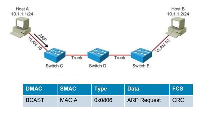
If Host A does not have an entry for Host B in its ARP cache, it will ARP for the Host B MAC address.
