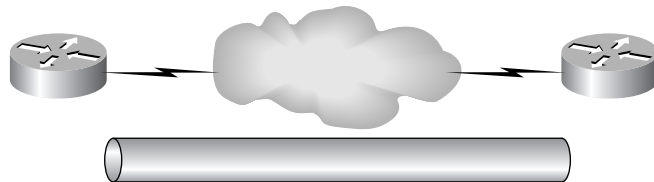
FIGURE 16.1 An IPSec tunnel
