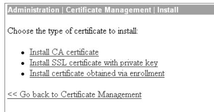
FIGURE 18.29 Installing the certificate on the concentrator
