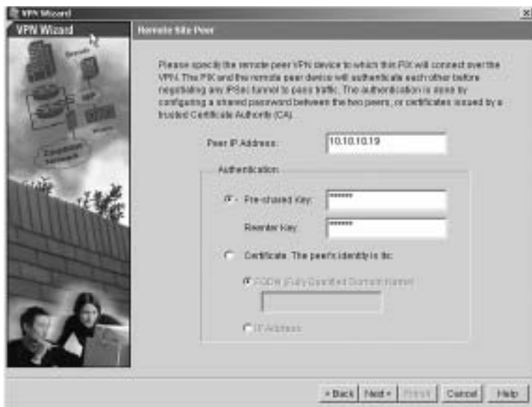
Figure 13-12 Remote Site Peer Window
