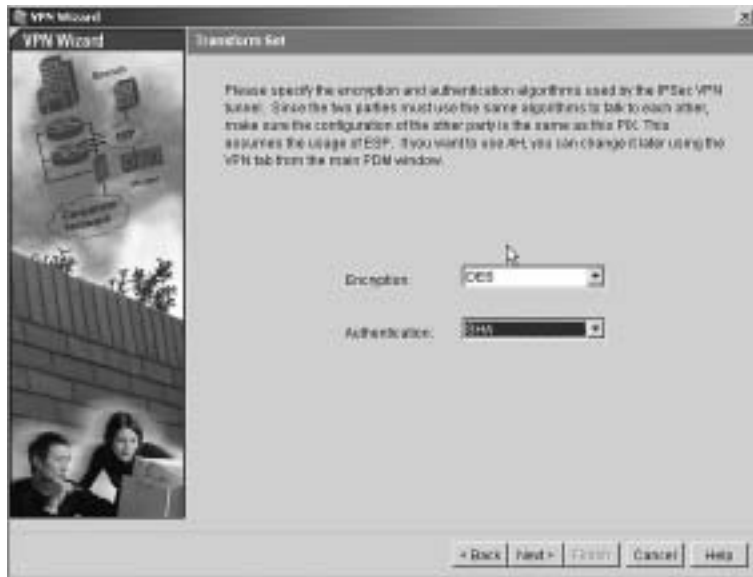
Figure 13-25 Transform Set Window
