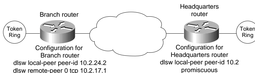
Figure 7-3 Example of dlsw local-peer and dlsw remote-peer commands.
