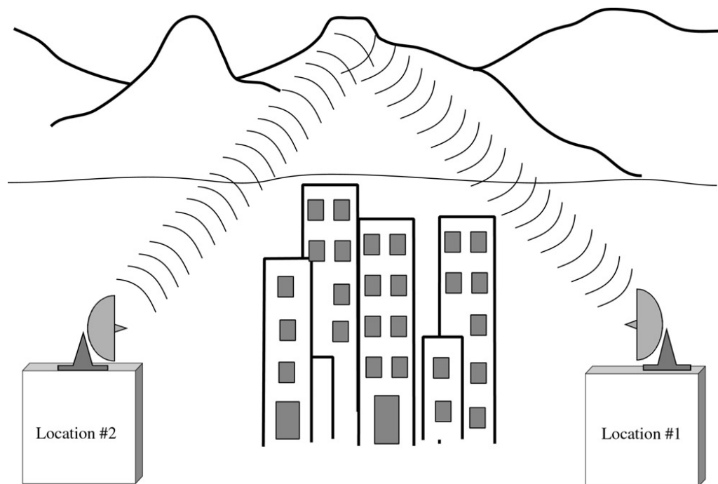
Figure 17-6: Obstacle gain uses a bounced signal off a natural obstacle, such as a mountain. If a repeater is needed, rental space is often available on other towers. This is true in long haul and also in localized communications. Renting space on an existing tower or a rooftop is not very dramatic. Leased space typically costs $200 per month per dish. Repeaters are shown in Figure 17-7.
