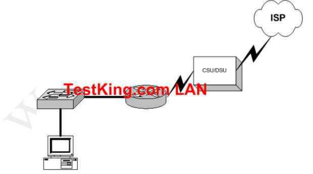
You are brand new to the company, and you are in the process of discovering the Testking network's topology. You have been given a Visio of the network diagram above. Based on this information, what conclusion can you make about the type of Testking Internet connection? (Select all that apply)
