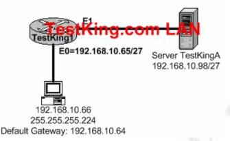
A new PC is installed on the LAN of the Testking1 router as shown above. This PC is unable to connect to the TestKingA server located on the Ethernet 1 network. What is the cause of this?
