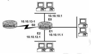
Router B has to forward an IP datagram to 10.10.10.10; which of the interfaces will be used by router B when forwarding this datagram?
