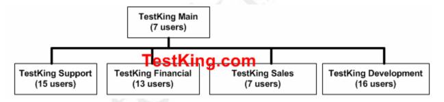
You are a systems administrator at TestKing and you've just acquired a new Class C IP network. Which of one of the subnet masks below is capable of providing one useful subnet for each of the above departments (support, financial, sales & development) while still allowing enough usable host addresses to meet the needs of each department?
