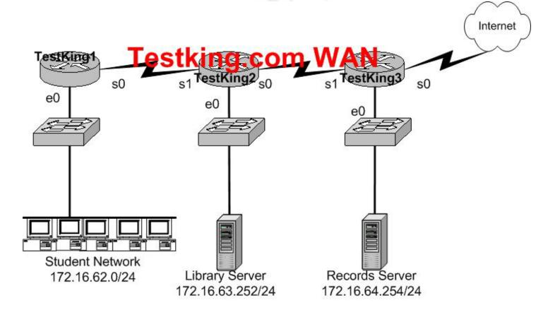
In the above network, an access list was created in order to prevent students and outsiders on the internet from changing student files in the Records Server, while still allowing other departments in the enterprise access. The access control list was applied to the e0 interface of the TestKing 3 router going outbound. Which two of the following conditions below were contained in the access control list? (Select two answer choices)
