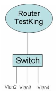
A switch has been configured for three different VLANs: VLAN 2, VLAN 3, and VLAN 4. For the purposes of communication between VLANs a router is to be added. Host from one VLAN should be able to reach the hosts in the other VLANs. Based on this requirement, what type of connection is acceptable between the router and switch?
