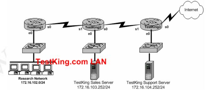
You are a network security consultant and you've been contracted to prevent users on the Research Network and general Internet surfers from accessing the TestKing Support server. However, you must allow access to all the other TestKing users. So you create an access control list called research\_network which contains the following lines:
