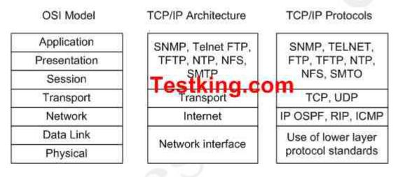
TCP/IP's architecture does not use the presentation and session layers. The application layer protocols use the transport layer services directly. The OSI transport layer provides connection-oriented service; in TCP/IP, this service is provided by TCP. TCP/IP also provides connectionless service in the transport layer with UDP.
