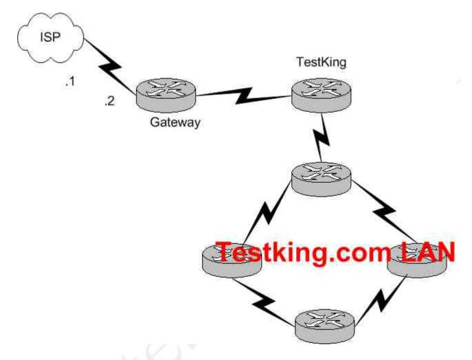
The ISP assigned you the class CIP address 207.134.6.0/30 for this Internet connection. A default route to the Internet should be set up. Which of the following are acceptable ways to configure this on the Gateway router? (Select all that apply)
