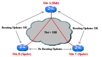
Figure 2: Split-horizon does not allow remote sites to send routing updates to each other.
