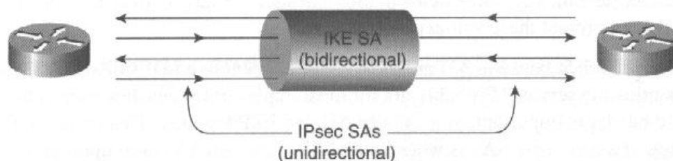
Figure 7-5 A Single IKE SA Acts as a Secure Management Channel for IPsec SAs
